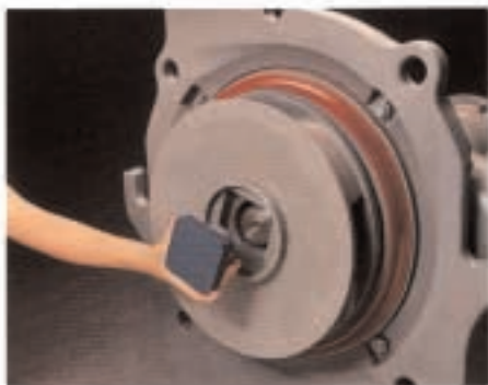
19. Place the runner on the shaft and secure with the runner bolt.
