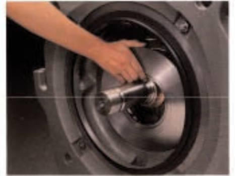
12. Place the die ring holder over the shaft so that it seats flush with the front bearing cap.
