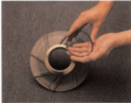
10. Place the shaft sleeve o-ring in the inner bore of the shaft sleeve.
