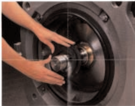
13. Seat the check valve diaphragm into the groove on the die ring holder. Be sure that the die ring is seated properly.
