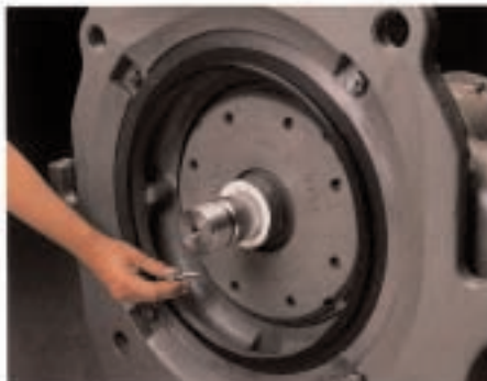
16. Attach the front die ring to the front bearing cap.
