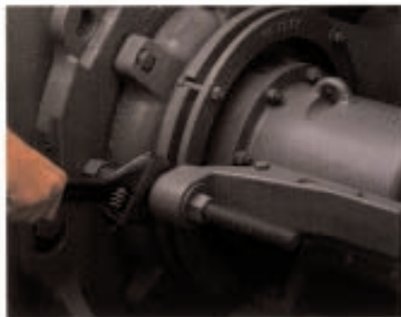
24. Adjust the runner clearance with the draw bolt assembly. Once runner is adjusted properly, securely tighten long cylinder to the frame.
