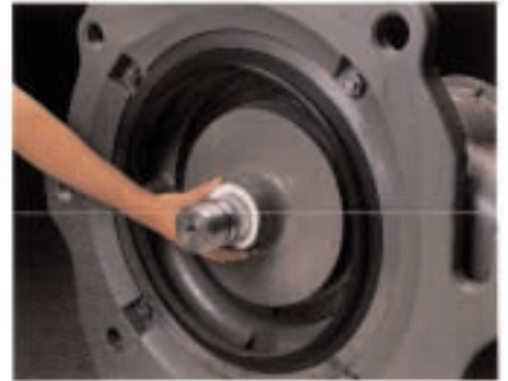
15. Slide the expeller onto the shaft and seat against the rear die ring.
