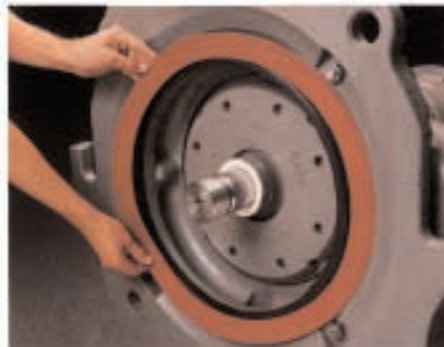
17. Place the intake chamber gasket on the intake chamber.
