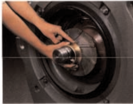
11. Slide the shaft sleeve onto the shaft and tighten with set screws. Set screws must seat properly on the flat area of the shaft.
