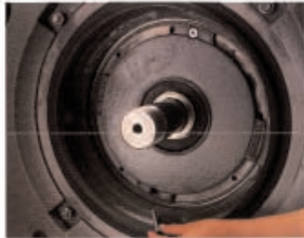
14. Attach the rear die ring to the front bearing cap.
